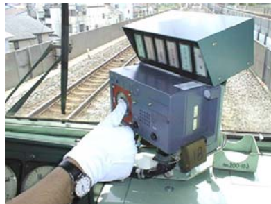
Figure 3: Train Protection System
